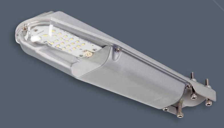
New generation energy saving and Environment-friendly long life LED street lights made up of pressure die-cast aluminium housing with high power LED as lighting source and lens embedded PC cover having TOP Opening seperate driver compartment with IP65 protection and impact resistance of IK07.
