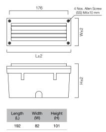
All dimensions are in mm Tolerance: ± 2 mm
